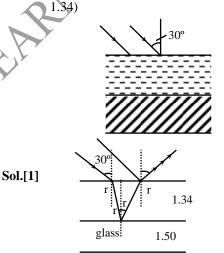
Condition for constructive interference
