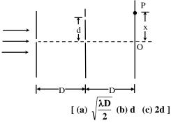
**Q.14** Figure shows three equidistant slits being illuminated by a monochromatic parallel beam of light. Let  $BP_0 - AP_0 = \lambda/3$  and  $D \gg \lambda$ . (a) Show that in this case  $d = \sqrt{2\lambda D/3}$ . (b) Show that the intensity at  $P_0$  is three times the intensity due to any of the three slits
