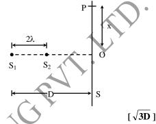
Q.13 Consider the arrangement shown in figure. The distance D is large compared to the separation d between the slits. (a) Find the minimum value of d so that there is a dark fringe at O. (b) Suppose d has this value. Find the distance x at which the next bright fringe is formed. (c) Find the fringe-width.
