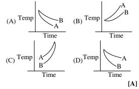
Rate of cooling is  $\propto \frac{1}{\text{radius}}$  so A is faster. Sol.
