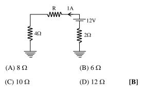
Q.31 In the circuit, the value of R is so chosen that thermal power generated in it is maximum, then value of R is –
