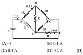
Q.30 In the circuit shown in figure the value of R is-
