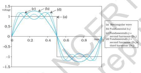
second harmonic  $(2v_0)$  + third harmonic  $(3v_0)$ , are shown in the same figure to illustrate this fact. It is clear that to reproduce the rectangular wave shape exactly we need to superimpose all the harmonics  $v_0$ ,  $2v_0$ ,  $3v_0$ ,  $4v_0$ ..., which implies an infinite bandwidth. However, for practical purposes, the contribution from higher harmonics can be neglected, thus limiting the bandwidth. As a result, received waves are a distorted version of the
