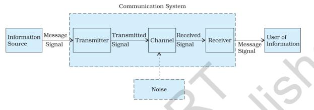
FIGURE 15.1 Block diagram of a generalised communication system
