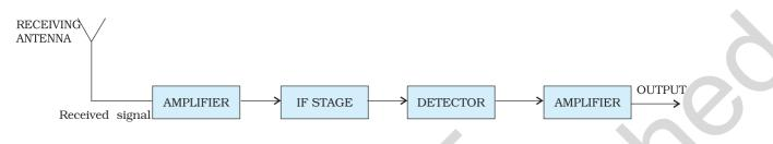
FIGURE 15.12 Block diagram of a receiver.
