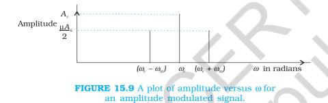
As long as the broadcast frequencies (carrier waves) are sufficiently spaced out so that sidebands do not overlap, different stations can operate without interfering with each other.
