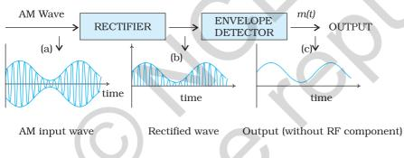
FIGURE 15.13 Block diagram of a detector for AM signal. The quantity on y-axis can be current or voltage.
