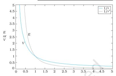
**FIGURE 2.4** Variation of potential V with r [in units of  $(Q/4\pi\varepsilon_0)$  m<sup>-1</sup>] (blue curve) and field with r [in units of  $(Q/4\pi\varepsilon_0)$  m<sup>-2</sup>] (black curve) for a point charge Q.
