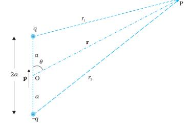
**FIGURE 2.5** Quantities involved in the calculation of potential due to a dipole.
