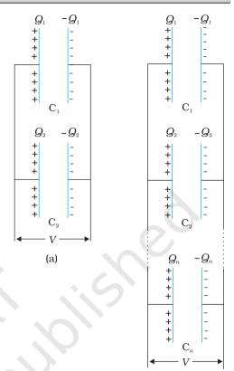
FIGURE 2.28 Parallel combination of (a) two capacitors, (b) n capacitors.
