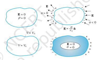
**FIGURE 2.19** Some important electrostatic properties of a conductor.
