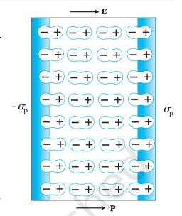
**FIGURE 2.23** A uniformly polarised dielectric amounts to induced surface charge density, but no volume charge density.
