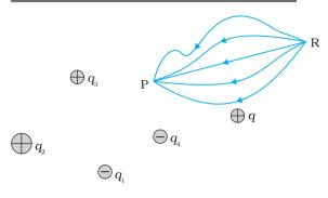
**FIGURE 2.2** Work done on a test charge q by the electrostatic field due to any given charge configuration is independent of the path, and depends only on its initial and final positions.
