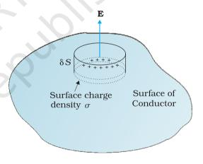
**FIGURE 2.17** The Gaussian surface (a pill box) chosen to derive Eq. (2.35) for electric field at the surface of a charged conductor.
