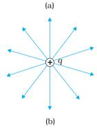
**FIGURE 2.9** For a single charge q (a) equipotential surfaces are spherical surfaces centred at the charge, and (b) electric field lines are radial, starting from the charge if q > 0.
