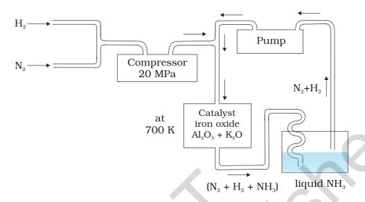
Fig. 7.1 Flow chart for the manufacture of ammonia
