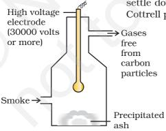
Fig. 5.15: Cottrell smoke precipitator
