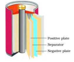
Another important secondary cell is the nickel-cadmium cell (Fig. 3.11) which has longer life than the lead storage cell but more expensive to manufacture. We shall not go into details of working of the cell and the electrode reactions during charging and discharging. The overall reaction during discharge is:
