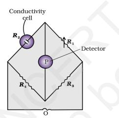
Once the cell constant is determined, we can use it for measuring the resistance or conductivity of any solution. The set up for the measurement of the resistance is shown in Fig. 3.5.
