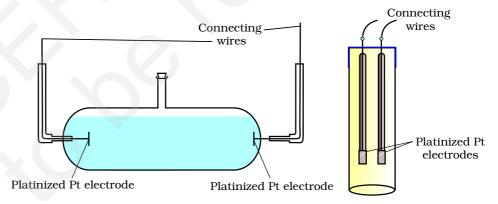
Basically it consists of two platinum electrodes coated with platinum black (finely divided metallic Pt is deposited on the electrodes electrochemically). These have area of cross section equal to 'A' and are separated by distance 'l'. Therefore, solution confined between these electrodes is a column of length l and area of cross section A. The resistance of such a column of solution is then given by the equation:
