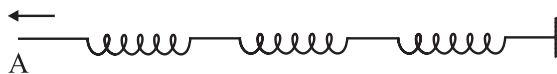
Fig. 15.1 A collection of springs connected to each other. The end A is pulled suddenly generating a disturbance, which then propagates to the other end.
