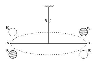
**Fig. 8.6** Schematic drawing of Cavendish's experiment.  $S_1$  and  $S_2$  are large spheres which are kept on either side (shown shades) of the masses at A and B. When the big spheres are taken to the other side of the masses (shown by dotted circles), the bar AB rotates a little since the torque reverses direction. The angle of rotation can be measured experimentally.
