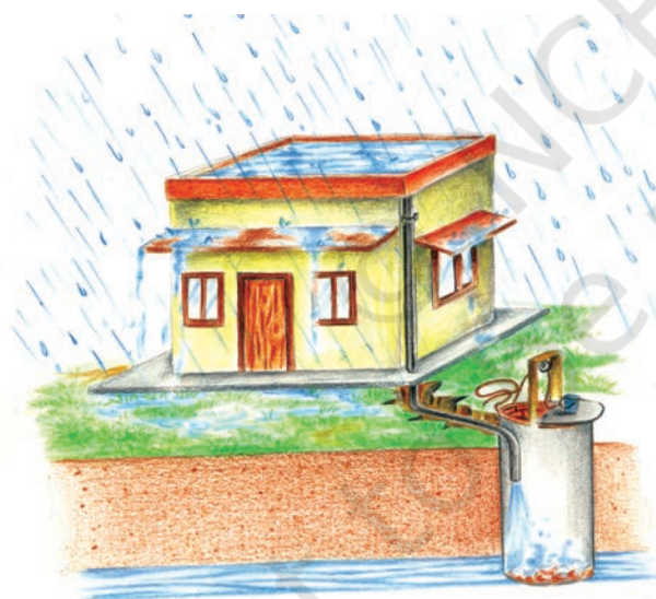
(b) Recharge through Abandoned Dugwell
