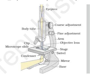
Fig. 5.1: Compound microscope
