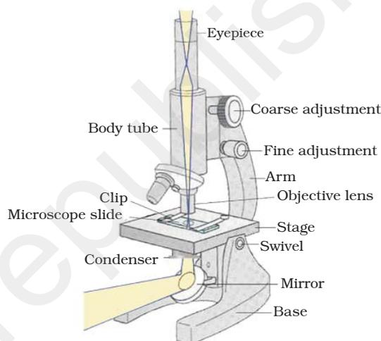
Fig. 5.1: Compound microscope
