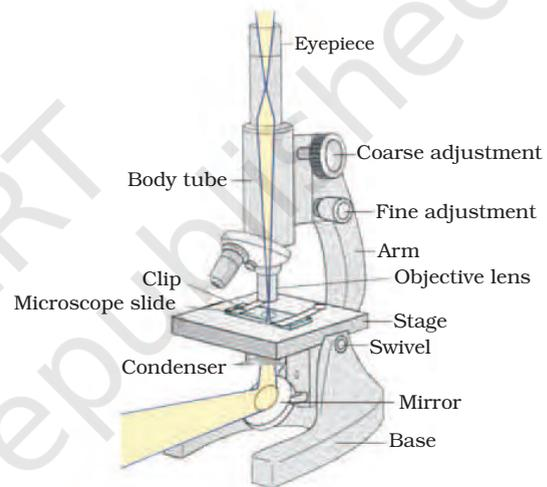
Fig. 5.1: Compound microscope
