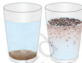
Fig. 9.2: Mixture of (a) Sand and water; (b) Sawdust and water
