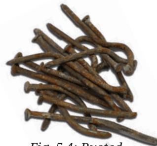
Fig. 5.4: Rusted iron nails
