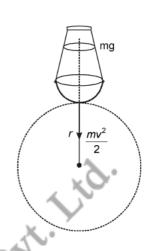
The necessary centripetal force required for the rotation of the man is provided by the normal force  $(F_N)$ .
