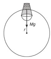
Let v be the velocity of the bucket at the top of the circular path. For rotating the bucket of water along a vertical circle, it requires a centripetal force  $Mv^2/r$ , where M is the mass of water and r, the radius of the circular path. The weight of the water provides the centripetal force and hence the water does not fall. In other words, the weight due to which the water can fall is used up in providing the necessary centripetal force.
