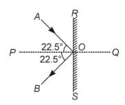
The horizontal components of velocities suffer no change. The vertical components of velocities are in the opposite directions
