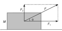
The acceleration will be produced along the direction of resultant force F. If the resultant force F makes an angle  $\theta$  with the direction of force  $F_1$ , then
