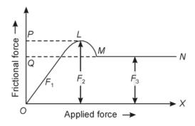
Therefore kinetic friction as once motion actually starts irregularities of one surface are not able to get locked into irregularities of another surface.
