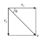
The resultant velocity (v) of the stone is given as:
