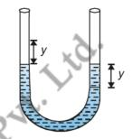
(b) (i) Let the liquid in the right arm be depressed through a distance y metre. Then the liquid in the left arm will rise through a distance y metre.
