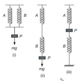
(b) As shown in the figure (ii), spring length is doubled and the weight mg will produce double the extension. If  $k_2$  is the spring factor of the combination, then
