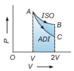
**S29.** The figure shows the P-V graphs for two samples of gas compresses from volume V to V/2 isothermally and adiabatically.
