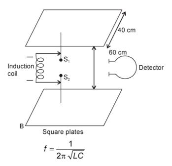
Oscillating magnetic field of e.m. waves induces an electric field in the ring of detector thus producing a spark across the air-gap in the ring.
