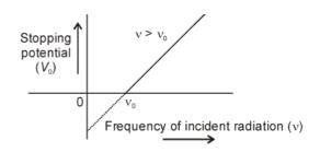
This equation is of the form y = mx + c which is the equation of straight line. Here slope is h/e and intercept is  $-\frac{\phi_0}{e}$ . From the intercept  $\left(-\frac{\phi_0}{e}\right)$  and the known value of e, value of work function  $(\phi_0)$  can be calculated.
