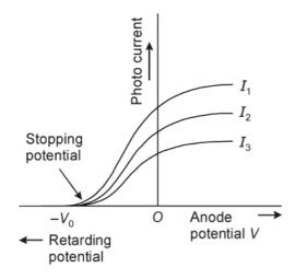
**S2.** The variation of photocurrent with the collector plate potential for different plate frequencies is shown below.
