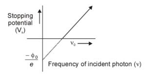
Thus, with the help of graph we can find out the value of stopping potential and threshold frequency.
