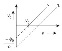
S9. Curves 1 and 2 correspond to similar materials while curves 3 and 4 represent similar materials, since the value of stopping potential for the pair of curves (1 and 2) and (3 and 4) are the same. For given frequency of the incident radiation, the stopping potential is independent of its intensity.
