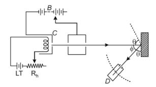
It was found experimentally that sharp peak of intensity of electron beam is obtained at 54 V accelerating potential and 50° scattering angle. By geometry, angle of glancing  $\theta$  is
