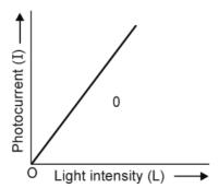
**S17.** Photoelectric effect: The phenomenon of ejection of electrons from a metal surface, when light of sufficiently high frequency falls upon it, is known as the photoelectric effect.
