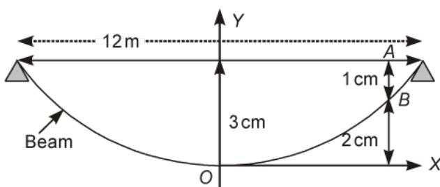
The equation of the parabola takes the form  $x^2 = 4ay$ . Since, it passes through  $\left(6, \frac{3}{100}\right)$ , we have
