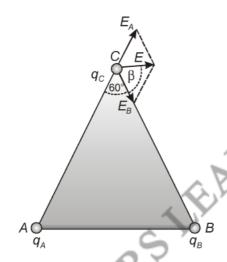
$$q_A = 60 \text{ StatC} = \frac{60}{3 \times 10^9} = 2 \times 10^{-8} \text{ C}$$
