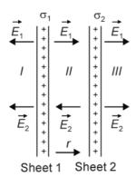
In the region I: Electric field due to charge sheet 1,
