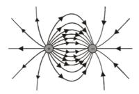
**S25.** The electric dipole moment of a dipole is equal to the product of either charge (q) and the vector  $\stackrel{\rightarrow}{2a}$  (separation) between the two charges. It is denoted by  $\stackrel{\rightarrow}{p}$ . Thus,
