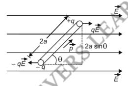
Two equal and opposite forces  $+ q\vec{E}$  and  $- q\vec{E}$  act on its two ends and constitute a couple. The torque exerted by the couple is given by
