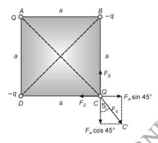
can be zero, if charge at the points B and D are negative in nature. Then, the force  $F_A$ ,  $F_B$  and  $F_D$  will act on the charge Q at point C as shown in the above figure.
