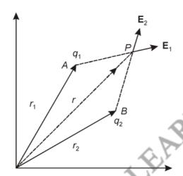
Electric field intensity at point P due to  $q_1$ ,
