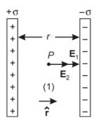
By Gauss's law, it can be proved that electric field intensity due to a uniformly charged infinite plane sheet at any nearby is given
