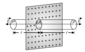
By symmetry, electric field points outward normal to the sheet. Also, it must have same magnitude and opposite direction at two points P and P' equidistant from the sheet and on opposite sides. We choose cylindrical Gaussian surface of cross sectional area A and length 2r with its axis perpendicular to the sheet.
