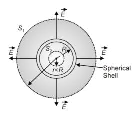
(a) When point *P* lies outside the spherical shell: The total charge q inside the Gaussian surface  $S_1$  is equal to the charge on the spherical shell.
