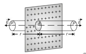
By symmetry, electric field points outward normal to the sheet. Also, it must have same magnitude and opposite direction at two points P and P' equidistant from the sheet and on opposite sides. We choose cylindrical Gaussian surface of cross sectional area A and length 2r with its axis perpendicular to the sheet.
