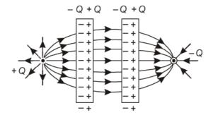
**Note:** Field lines must be perpendicular to the plates. Also, equispaced field lines exist between two plates as electric field between them is uniform.
