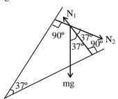
$$\frac{\text{mg}}{\sin(180^{\circ}-37^{\circ})} = \frac{N_2}{\sin(180^{\circ}-37^{\circ})}$$
