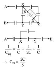
Q.25 If  $C_0$  is the capacitance between two adjacent plates, find the capacitance of the combination between A and B –
