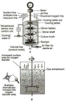
A-Simple stirred-tank bioreactor for continuous culture.
