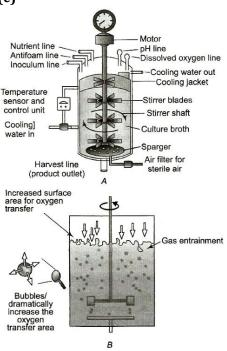
A-Simple stirred-tank bioreactor for continuous culture.
