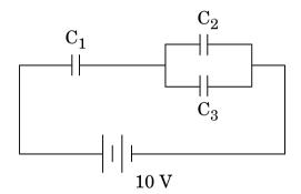
The figure shows a network of three capacitors  $C_1$  = 2  $\mu F$ ;  $C_2$  = 6  $\mu F$  and  $C_3$  = 3  $\mu F$  connected across a battery of 10 V. If a charge of 6  $\mu C$  is acquired by the capacitor  $C_3$ , calculate the charge acquired by  $C_1$ .
