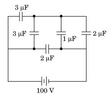
The figure shows a network of five capacitors connected to a 100 V supply. Calculate the total energy stored in the network.
