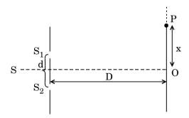
(c) In Young's double slit experiment, the slits are separated by 0.5 mm and screen is placed 1.0 m away from the slit. It is found that the  $5^{\text{th}}$  bright fringe is at a distance of 4.13 mm from the  $2^{\text{nd}}$  dark fringe. Find the wavelength of light used.
