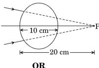
A point 'O' marked on the surface of a glass sphere of diameter 20 cm is viewed through glass from the position directly opposite to the point O. If the refractive index of the glass is 1.5, find the position of the image formed. Also, draw the ray diagram for the formation of the image.
