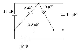
The figure shows a network of five capacitors connected to a 10 V battery. Calculate the charge acquired by the 5  $\mu F$  capacitor.
