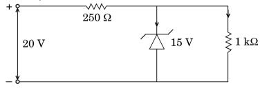
Give reason to explain why n and p regions of a Zener diode are heavily doped. Find the current through the Zener diode in the circuit given below : (Zener breakdown voltage is  $15\ V$ )
