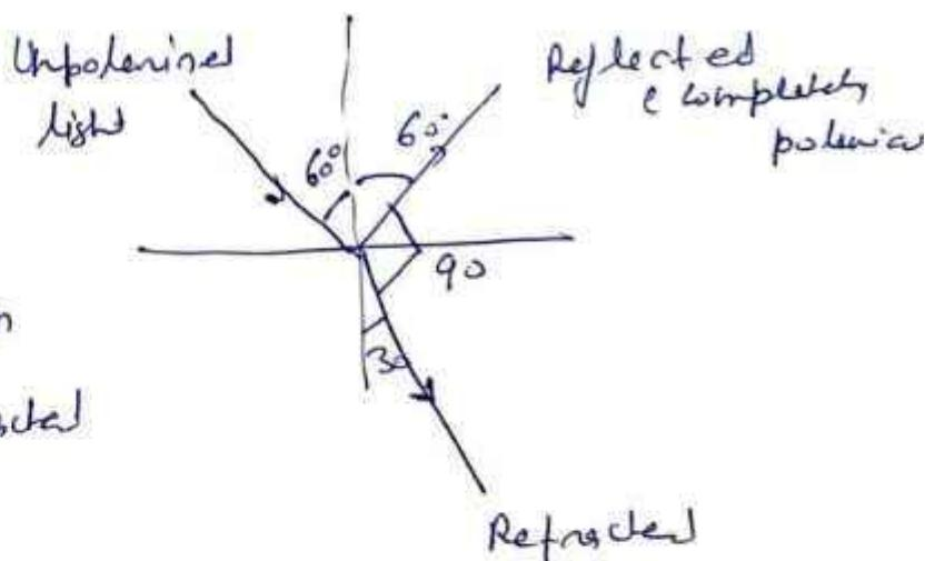
$$\text{angle of Refraction} = 180 - (90 + 60) \\ = 30^\circ$$
