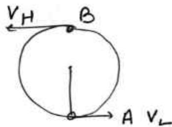
minimum velocity at A to complete the circle  $v = \sqrt{5gL}$
