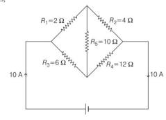
Now, if the 10  $\Omega$  wire is replaced with 15  $\Omega$  wire, the bridge still remains balanced. Hence, current drawn from battery will be 10 A.
