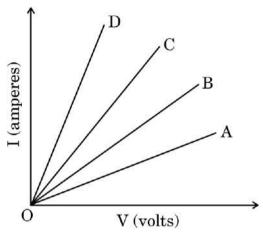
(a) Which one of the graphs represents the series combination of  $R_1$  and  $R_2$ ?
