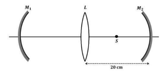
Q.10 In an experiment for determination of the focal length of a thin convex lens, the distance of the object from the lens is 10 ± 0.1 cm and the distance of its real image from the lens is 20 ± 0.2 cm. The error in the determination of focal length of the lens is n %. The value of n is \_\_\_\_\_\_.
