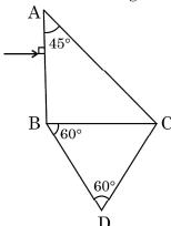
The critical angles for the two prisms with respect to air are  $41.1^{\circ}$  and  $45^{\circ}$  respectively. Trace the path of the ray through the combination.
