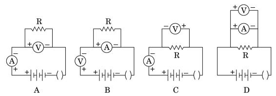
Which one of the following is the correct set-up for studying the dependence of the current on the potential difference across a resistor and why?
