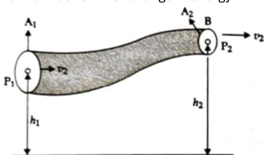
$$(P_1 - P_2) = \rho g(h_2 - h_1) + \frac{\rho}{2} (v_2^2 - v_1^2)$$
