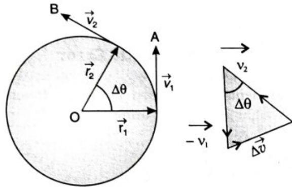
$$\text{Angular speed } \omega = \frac{\Delta\theta}{\Delta t} \dots (1)$$
