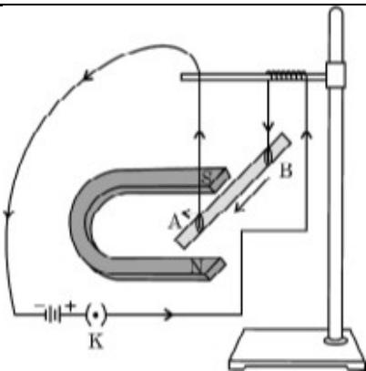
**A.** i. In the above experimental set up, when current is passed through the rod, it gets displaced towards the left. What will happen to the displacement if the polarity of the magnet and the direction of current both are reversed?
