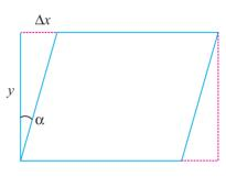
$\therefore$  Angle of shear  $\alpha$  is given by
