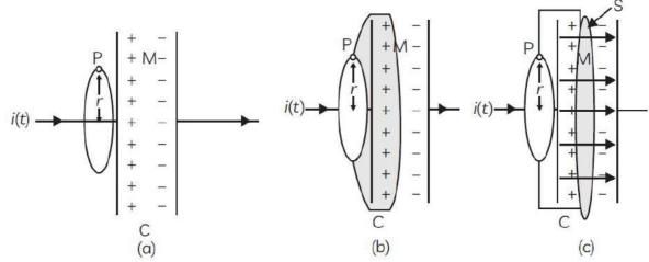
$I_D = \varepsilon_0 \frac{d\phi_E}{dt}$ , where  $\frac{d\phi_E}{dt}$  is the rate of change of electric flux between the plates of given capacitor.
