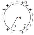
(a) If q > 0 and is displaced away from the centre in the plane of the ring, it will be pushed back towards the centre.
