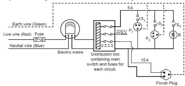
36. Study the schematic diagram of one of the common domestic circuits given below:
